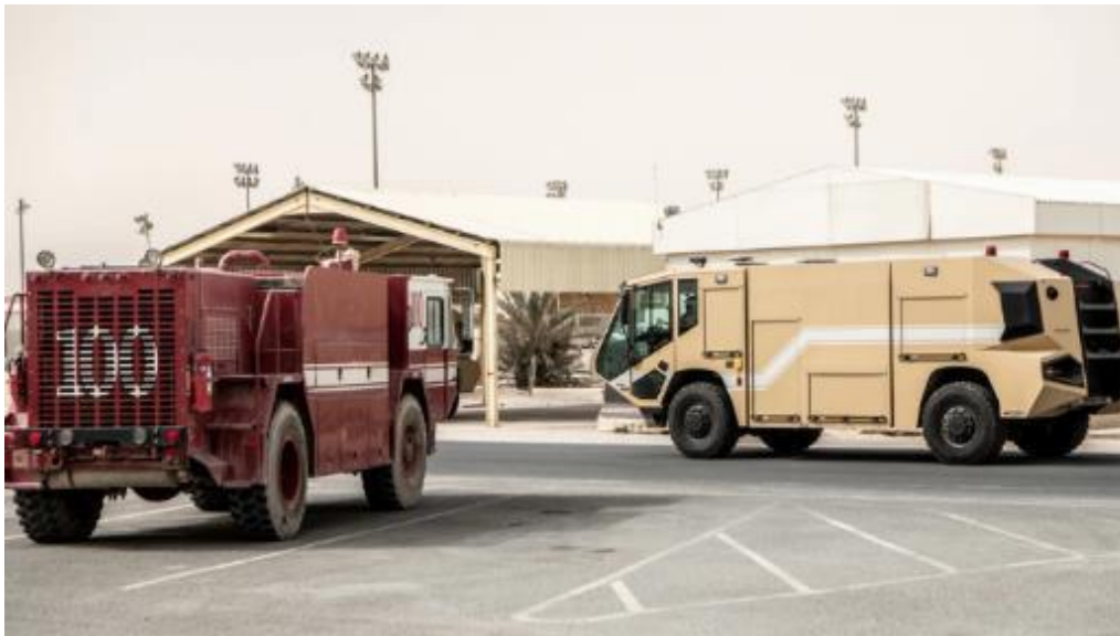
Figure 3: P-19C Firetruck replaces the older (red) P-19 legacy truck for contingency operations
