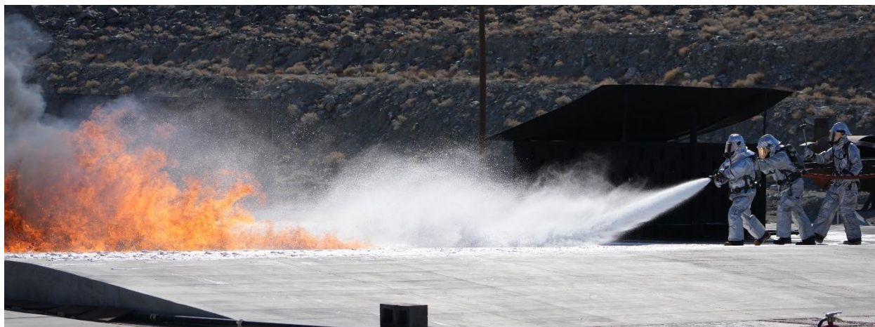
Fig. 4.5-4 – Roll-on Foam Application
