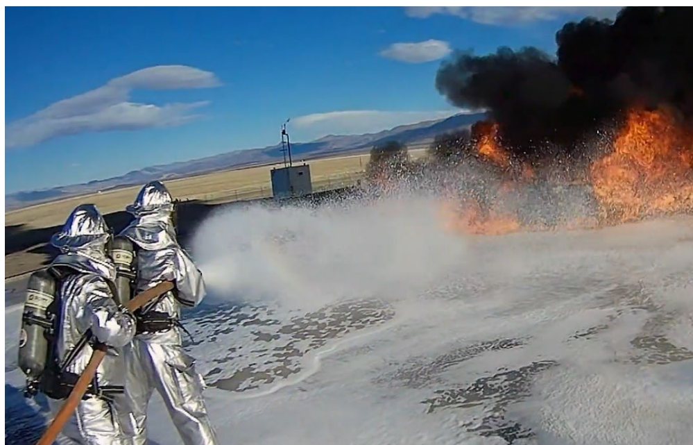
Fig. 4.5-3 – Rapid Foam Breakdown Shortly After Application
