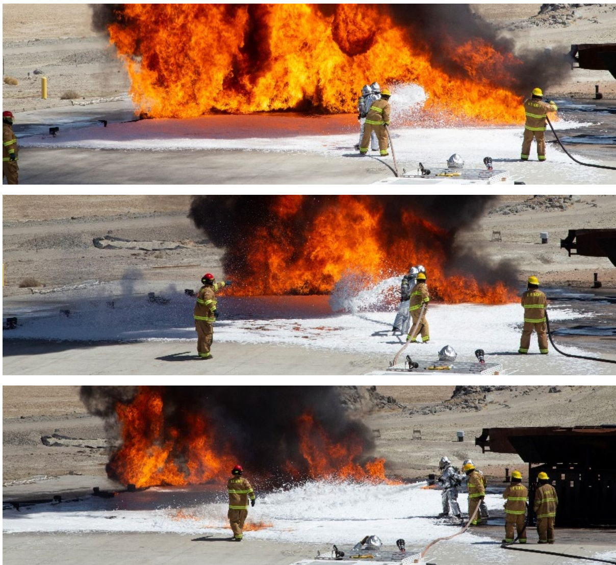
Fig. 4.2-2 – Openings in F3 Aspirated Foam Blanket
