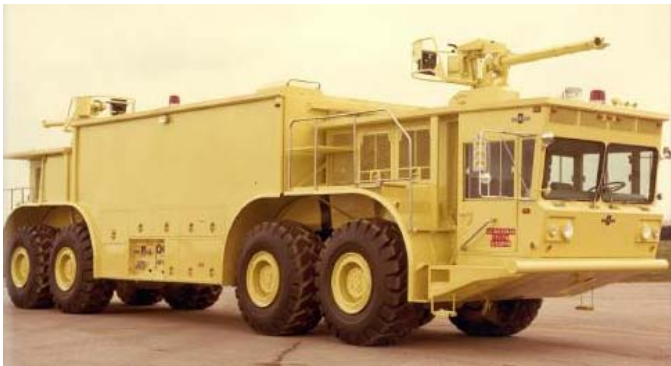
Tom Kelly's photo of the 1979 Oshkosh P-15 at Seymour Johnson AFB near Goldsboro, N.C. With a gross weight of 130,860 lbs, the P-15 is 542 inches in length, 163½ inches high, and 122 inches wide. Foam or water discharge capacity is 2,400 gpm.
