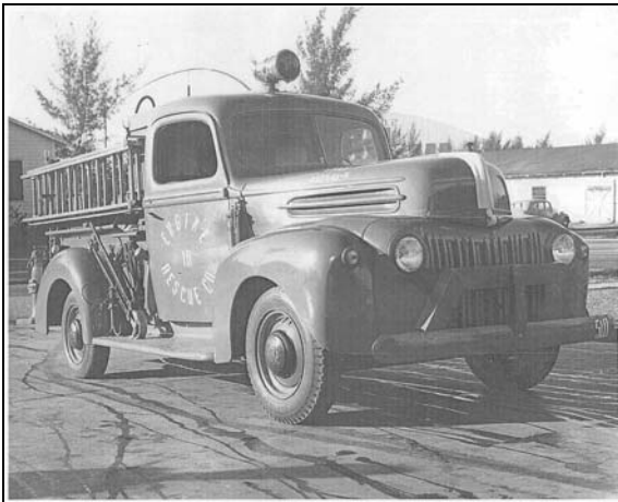
The first Air Force Aircraft Crash Rescue Truck, Engine 10, Rescue Company, MacDill AFB, Tampa, Florida, 1947-1959. Chief Frank Joseph built this unit on a half-ton Ford chassis. The elite rescue crew was credited with saving many aircraft crew members. Chief Lloyd W. Garner was crew chief of this specialized unit and received the Soldier's Medal, along with the rest of his crew, for rescuing a flight crew from a burning aircraft.
