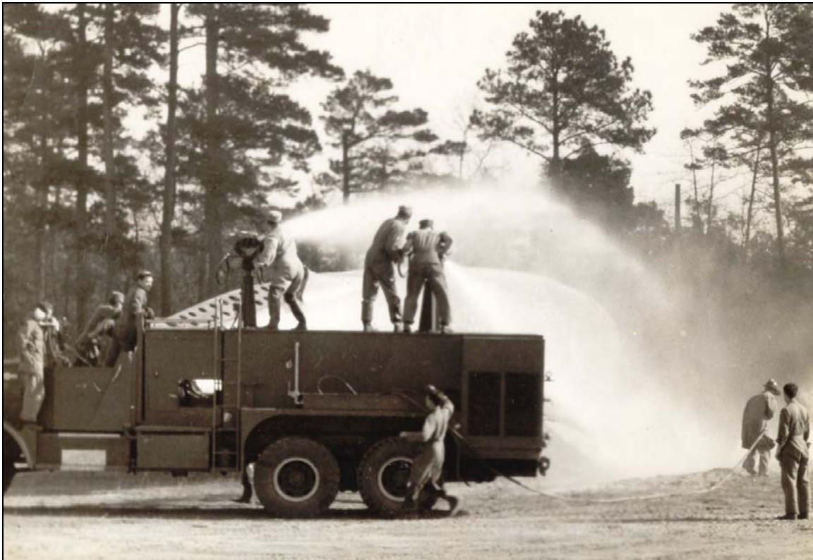
Fire fighting school at Shaw AFB, South Carolina, 1949. The Class 155 crash truck in operation is discharging high-pressure water fog on a training fire. Chief Paul Odell conducted the training for military fire fighters.
