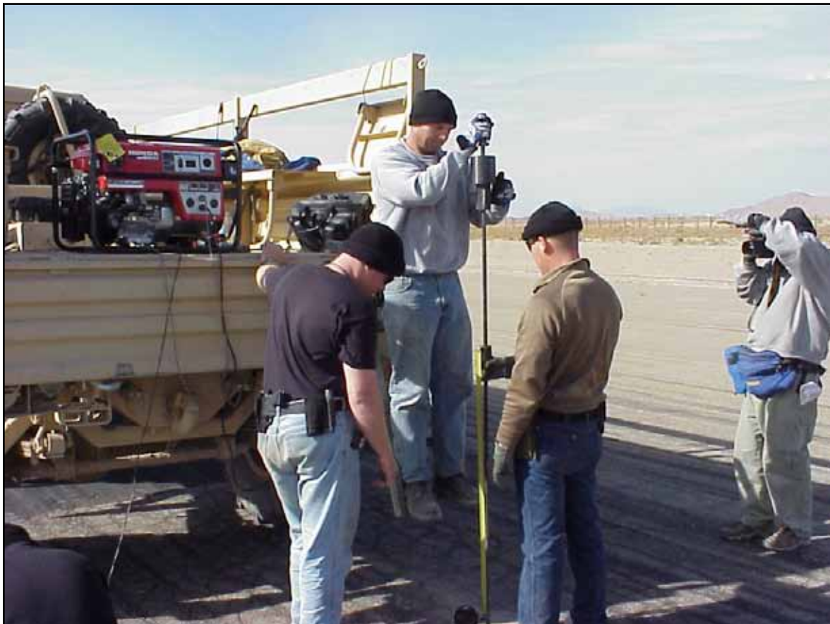
The AFCEA Airfield Pavement Evaluation Team uses a dynamic cone penetrometer to evaluate a runway at Kandahar, Afghanistan.
