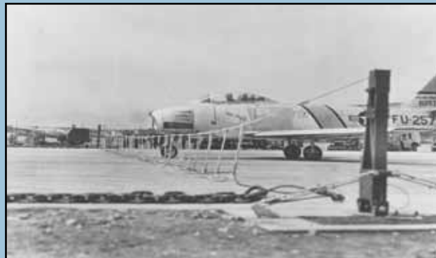
The Air Force tests a MA-1A aircraft arresting system using an F-86 "Sabre" jet at a base in Japan. This system used heavy ship's anchor chain to slow down the aircraft.
