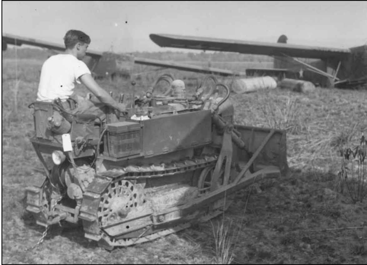
An airborne aviation engineer uses a tractor he just unloaded from one of the Waco gliders in the photo.
