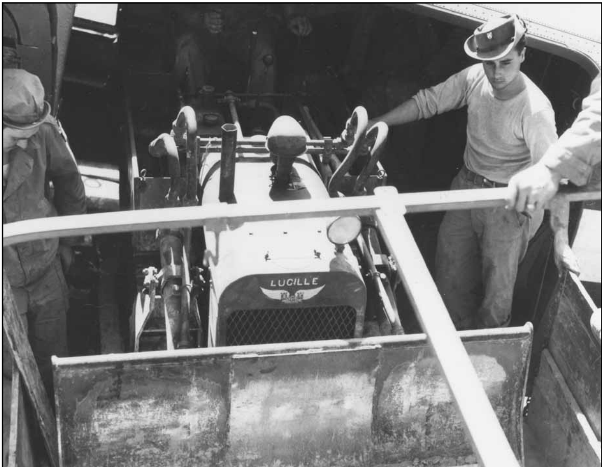
Airborne aviation engineers unload "Lucille," a specially designed tractor, from a C-47 at Tamu, Burma.
