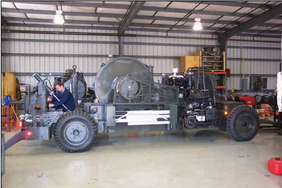
A Tyndall CEMIRT technician puts the finishing touches on a refurbished Mobile Aircraft Arresting System.
