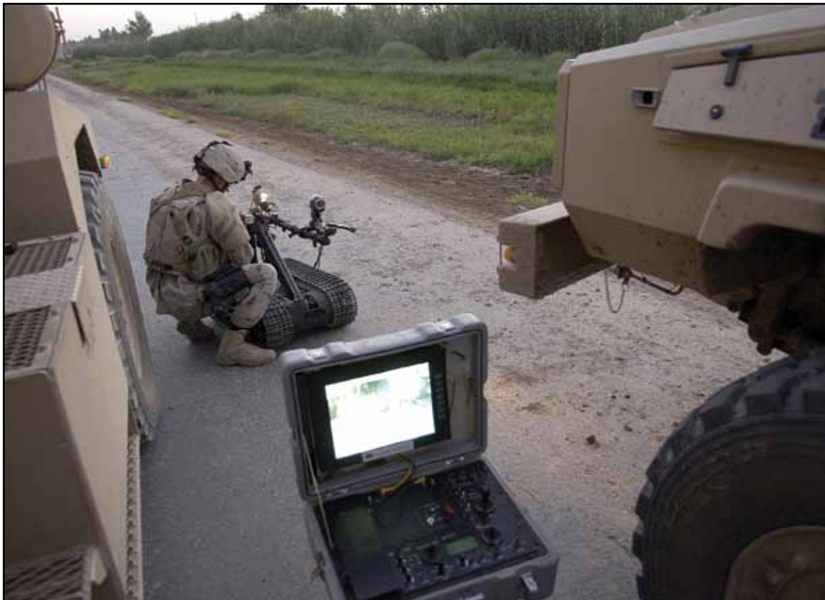
An EOD technician prepares a Talon robot before sending the robot to inspect a possible improvised explosive device.
